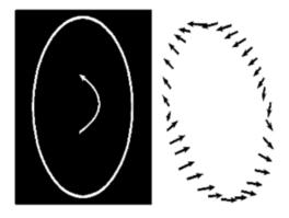
Note. The normal velocity components (right) of the edge of a rotating ellipse (left).
