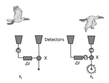
*Note.* The filter has two spatially separate detectors. The output of one of the detectors is delayed and the two signals are multiplied. The output is tuned to speed. Many detectors tuned to different speeds are required for the true speed of a pattern, and the difference of pairs of detectors tuned to different directions is taken (Reichardt, 1959; Robbins, 2004).
